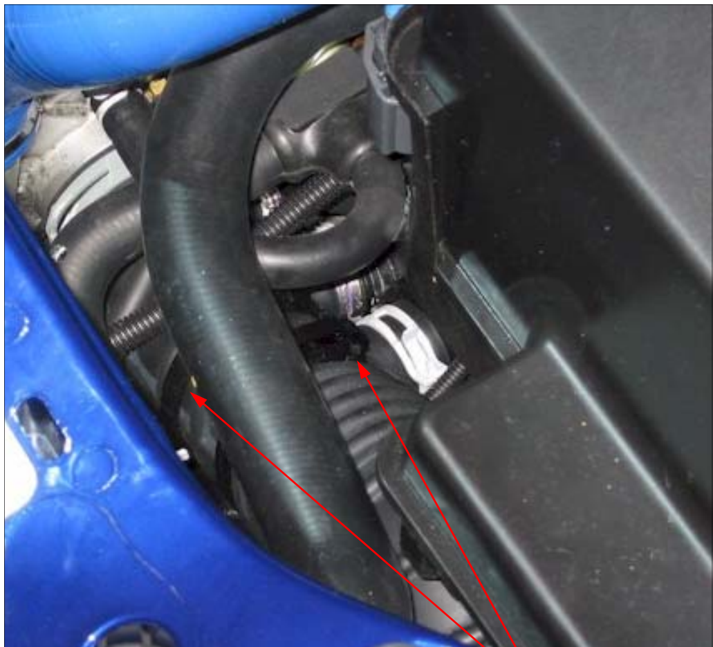
80 + 65 Clips fitted to the Air Induction Hose
